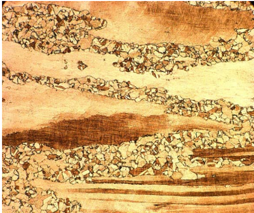
Figure 1: Duplex grain structure of standard hot-worked copper beryllium
