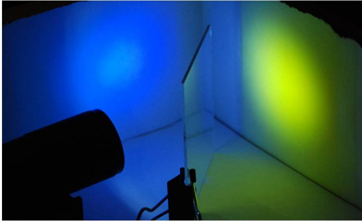
Figure 2. Dichroic coating reflects blue and transmits complimentary color yellow. (Photo by author S. Pellicori).
