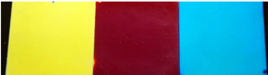
Figure 3. Colored reflectors are produced by absorbing the transmitted complimentary colors. (Photo by S. Pellicori).
