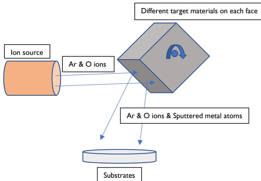
Figure 1. Illustration of the components of an ion beam sputtering (IBS) system. Up to four materials can be selected by rotation of the target cube. The substrate holder is rotating during deposition for the best uniform coverage.
