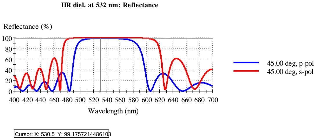
Figure 2. Reflectance at 45° AOI for the design (HL)<sup>12</sup>.
