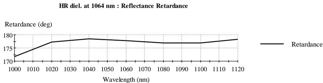
Figure 7. Retardance of a QW 1064 nm reflector with design (HL)<sup>12</sup>.
