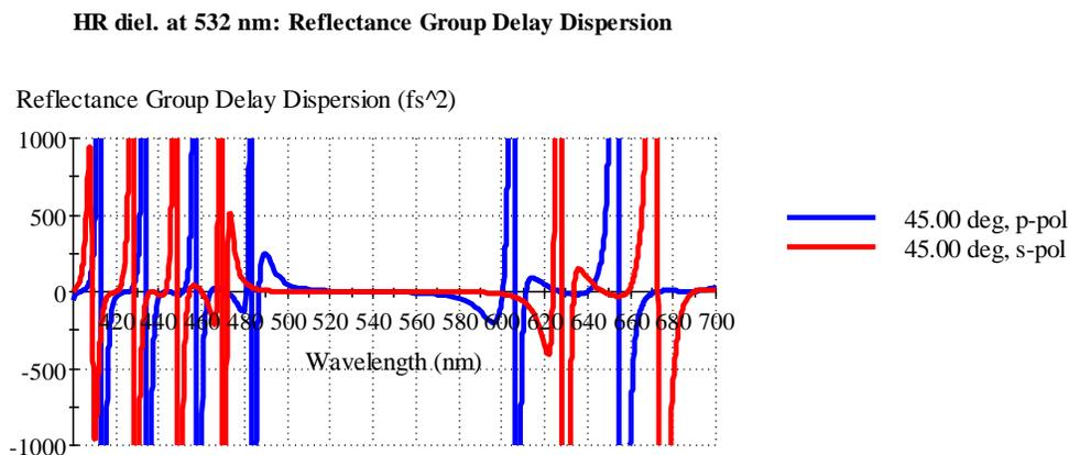
Figure 6. Group delay dispersion (GDD) changes rapidly away from the 532 nm center wavelength for the reflector of Figure 2.
