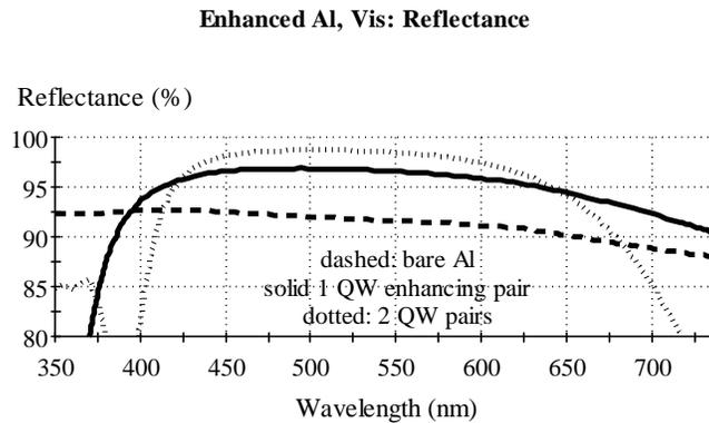
Figure 1. Al reflector protected by a single layer of SiO and enhanced by one and two QW pairs of TiO<sub>2</sub> and SiO<sub>2</sub>. Dielectric layers increase reflectance but narrow the wavelength coverage.
