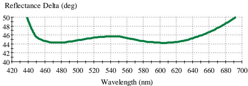
Figure 5. 45° retardance at a TIR surface in SF 56 glass.
