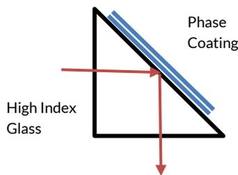
Figure 3. Configuration that produces controlled retardance at internal reflection.
