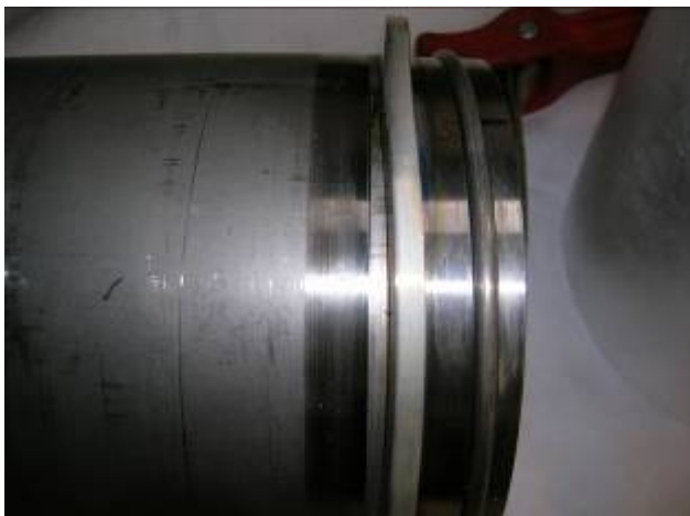
Figure 4. Deformed Welded Retaining Ring without Sleeves
