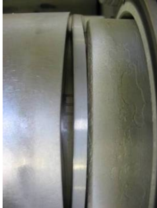
Figure 5. Deformed Welded Retaining Ring with Sleeves Mounted
