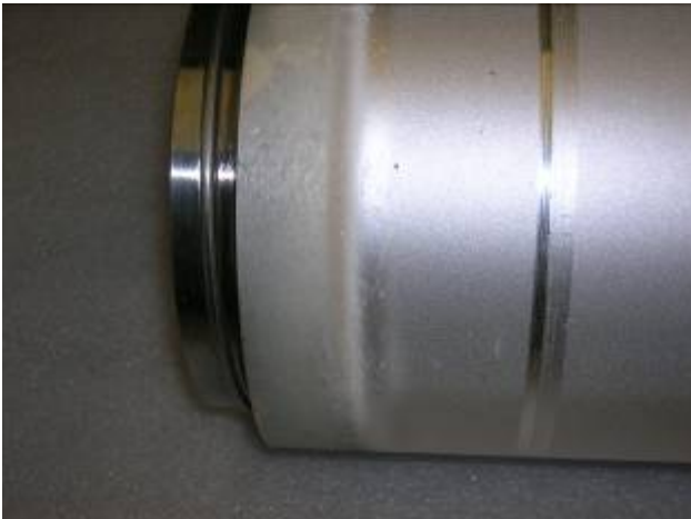
Figure 1. Thermocouple Contact Point
