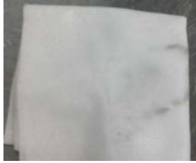
Fig. 9 Carbon residue after wiping a Au melt made from organic contaminated Au source material
