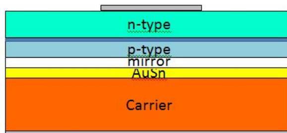
Fig. 1. Schematic of a LED structure where a AuSn solder layer is used for attachment to a carrier.
