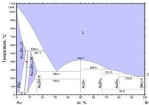
We studied the functioning of this solder in compound semiconductor applications, considering the entire soldering system and its effect on the chemistry, wetting and strength of the solder. A careful analysis of these factors indicates an ideal deposited solder film that is slightly tin rich when deposited onto a pure gold layer. When the solder is tin rich and the adjoining surfaces are pure gold, the gold will be dissolved into the solder taking the
