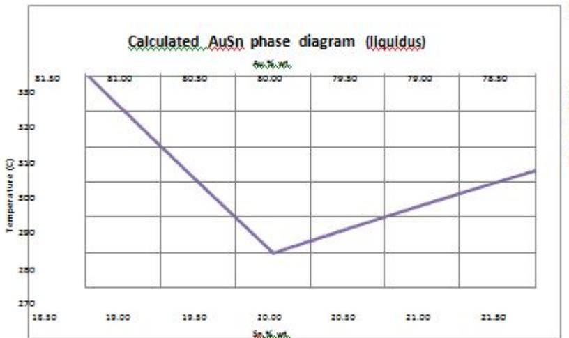
Figure 3. AuSn phase diagram near the eutectic composition.
