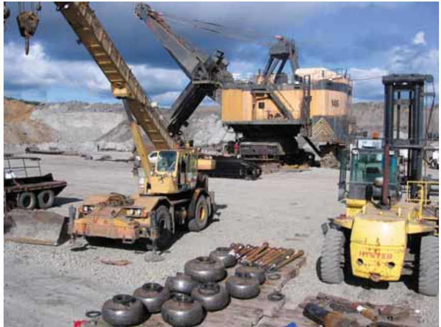
Figure 2: Mine maintenance pad with shovel shown in the distance. Load rollers with used ToughMet bushings from right side of shovel are on the pallet in the foreground.
