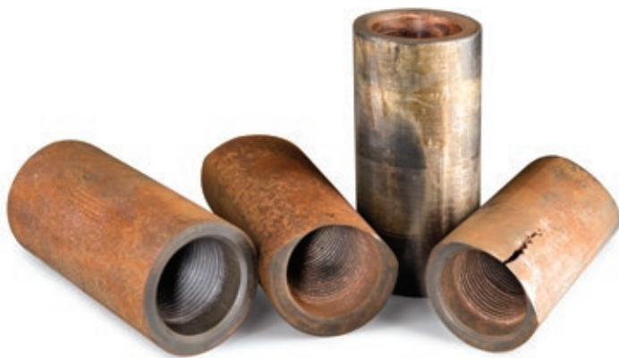
One ToughMet coupling (vertical) with three conventional couplings after 600 days in service.
