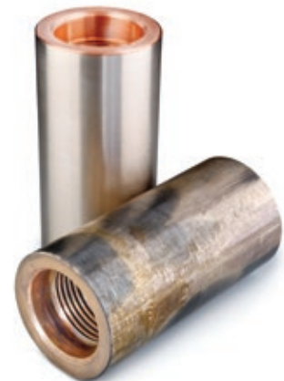
New ToughMet (vertical) coupling with ToughMet (horizontal) coupling after 600 days in service.
