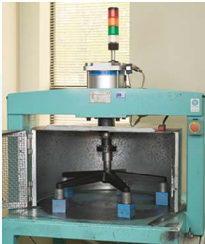
The Business and Institutional Furniture Manufacturer's Association (BIFMA) standards require chair bases withstand 2,500 lbs. ultimate load. RT Technology tests all bases to 3,000 lbs ultimate load.
