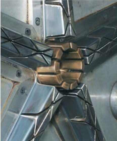
Injection Molding Machine: RT Technology's chair base mold with MoldMAX HH insert as seen at RT Technology
