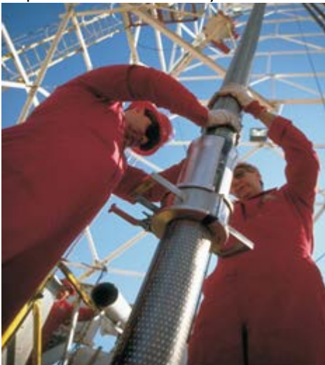
ToughMet 3TSI60U rod is used within the expansion tool for the ESS® system.
