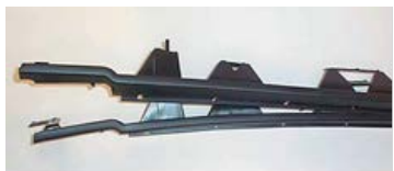
This photo shows two molded parts: the upper part shows a dimensionally conforming part molded at 49 seconds with P-20. The lower part shows deformation as a result of running the same tool at a reduced 37 seconds. Most steel tools are slowed down to mask the effect of poor heat transfer on the molding process. However, with its superior thermal properties, a MoldMAX HH tool was implemented in the design, ran at 37 seconds, and produced a part that was dimensionally accurate and conforming.
