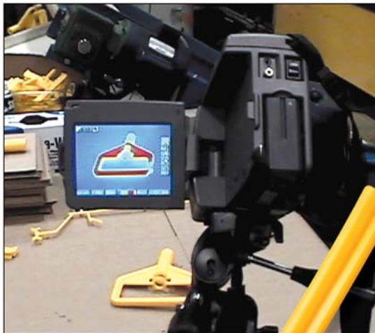
IR imaging captures a true picture of your mold's thermal performance
