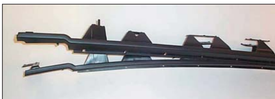
This photo shows two molded parts: the upper part shows a dimensionally conforming part molded at 49 seconds with P-20. The lower part shows deformation as a result of running the same tool at a reduced 37 seconds. Most steel tools are slowed down to mask the effect of poor heat transfer on the molding process. However, with its superior thermal properties, a MoldMAX HH tool was designed in, ran at 37 seconds, and produced a part that was dimensionally accurate and conforming.
