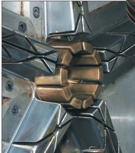
Injection Molding Machine - RT Technology's chair base mold with MoldMAX HH insert as seen at RT Technology.
