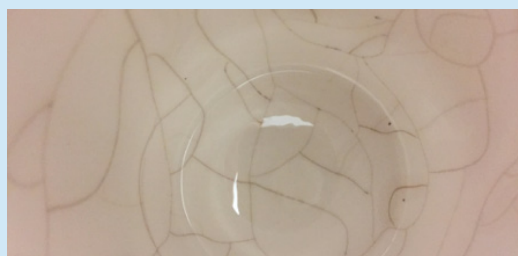
Figure 1. Crazing on Ceramic Surface. The inside of this coffee mug has a crazed appearance due to thermal cycling in an automatic dishwasher. This is why it is important to teach your children what the phrase “Hand wash only” means.
