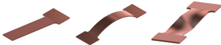
Figure 1. Comparison of the unit spring used for socket contacts. From left, cantilever beam, simply supported (arch) beam, torsion bar (louvered spring) contacts.
