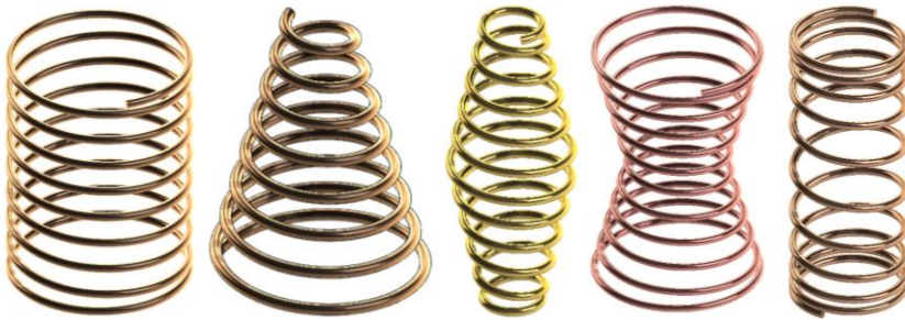
Figure 2. Various Types of Coil Springs. The boring spring on the far left is straight-sided and has constant pitch. The three constant-pitch springs in the middle are tapered into conical, barrel, and hourglass shapes, respectively. The spring on the far right is straight sided, but has variable pitch. Variable pitch springs may also be tapered, if required.
