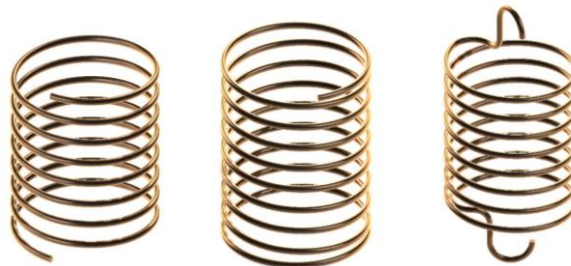
Figure 1. Coil Springs. The open-ended spring on the left is about as generic as a coil spring can get. The same spring is shown as a compression spring with closed ends in the middle, with the addition of flat, non-active coils at its top and bottom. On the right is the same spring as an extension spring, with hooks added to its top and bottom.
