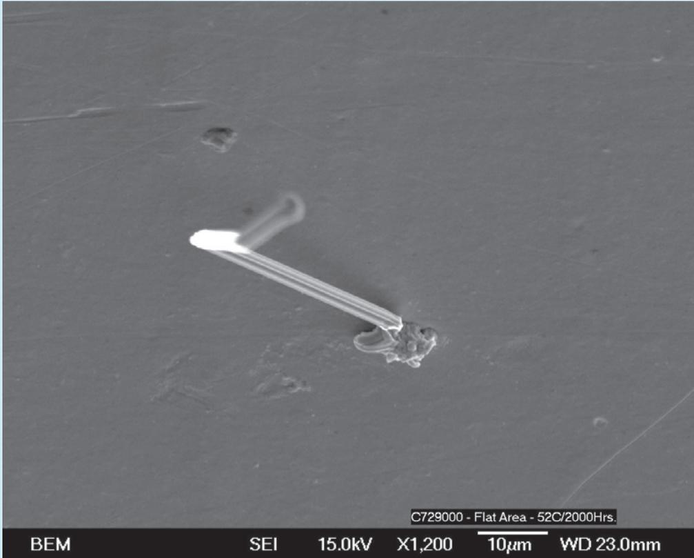
**Figure 1 – Secondary Electron Image (SEI) of a Tin Whisker Growing out of a Tin-Plated Surface.**
