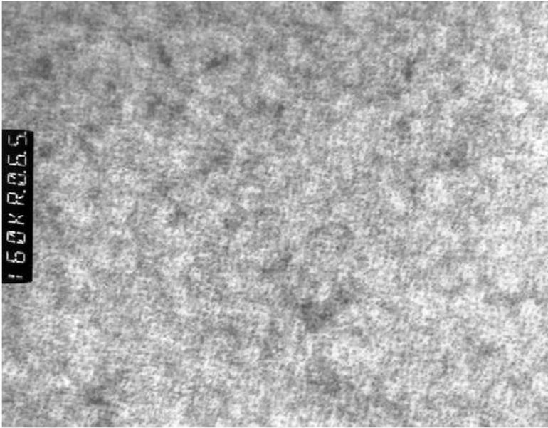
Transmission electron micrograph showing the spinodal structure in aged ToughMet 3 alloy, 160,000X (alternating waves of chemically different but structurally coherent atomic clusters of copper, nickel and tin present after spinodal decomposition.)
