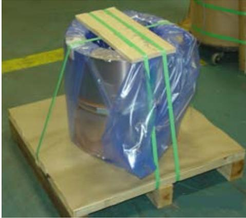
**Figure2. Coiled strip wrapped in plastic ready for international shipment.**
