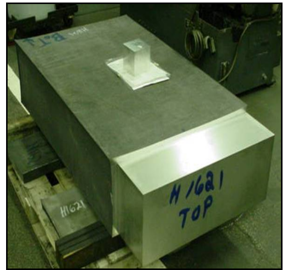
Fig 6 Partially machined HIPed blank
