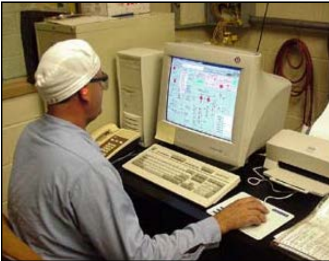
Fig 5 Control Console for Beryllium & Composites' HIP unit
