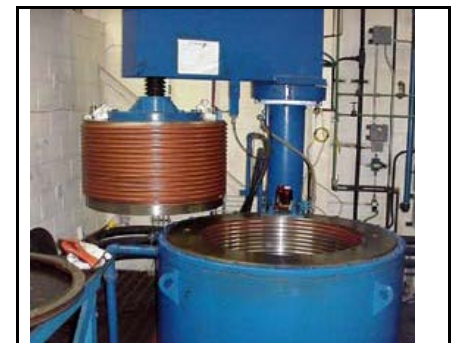
Fig 4 Beryllium & Composites 0 inch (760 mm) HIP unit.
