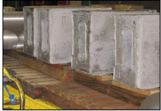
Fig 8 Direct HIPed beryllium blanks for mast mounted helicopter sight sensor supports
