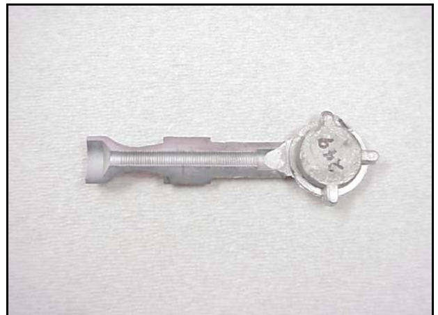
Figure 5 SSM Formed Parts for 30mm Bradley Fighting Vehicle Sabots
