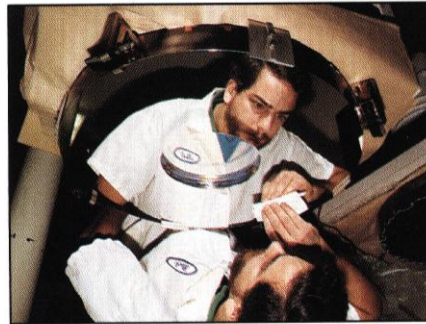
Polished mirror for RME system proved critical for bouncing laser beams off a satellite and hitting a ground target.
