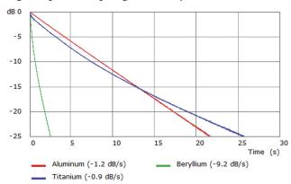
So, why does this happen? As detailed in our white paper on beryllium compression drivers<sup>1</sup>, the speed of sound in a solid material is a good indicator of acoustic performance, especially of resonant break-up modes due to diaphragm bending. The speed of sound likewise governs the bending frequency of a beam, or even a tuning fork (which is just two beams the same size).
