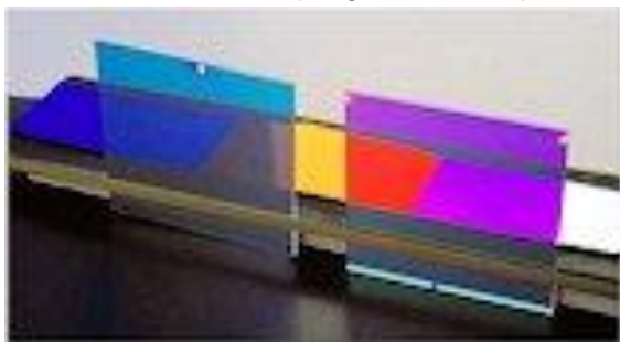
Depiction of coatings with the subtractive & additive combinations of colors produced by transmission through dichroic filters designed for the visible region.
