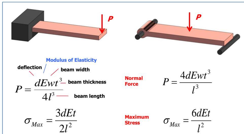
**Figure 2. Cantilever Beam vs Simply Supported Beam Spring Type and Relevant Equations for Rectangular Cross Sections.**
