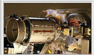
Astrium's NAOMI camera fitted with Materion multispectral arrays. Photo Credit: EADS Astrium, France
