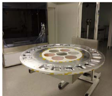
Coating fixture on the handling equipment.
