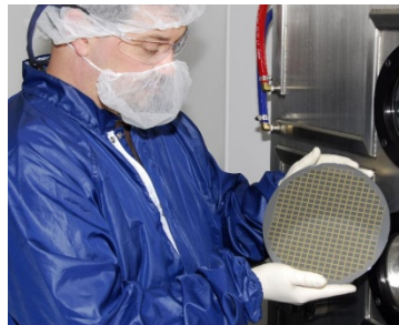
Patterned Low Defect Anti Reflective Coating on Wafer
