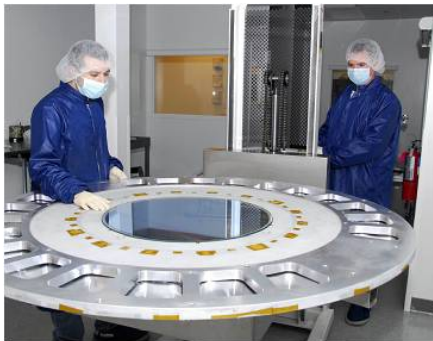
600 mm lens after coating
