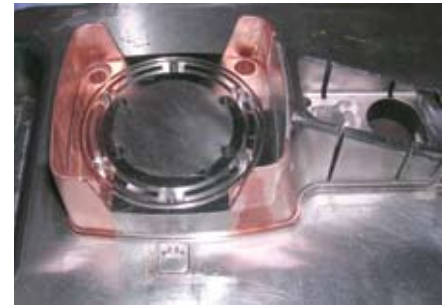
A typical application for CNS-V as an insert in a steel mold.
